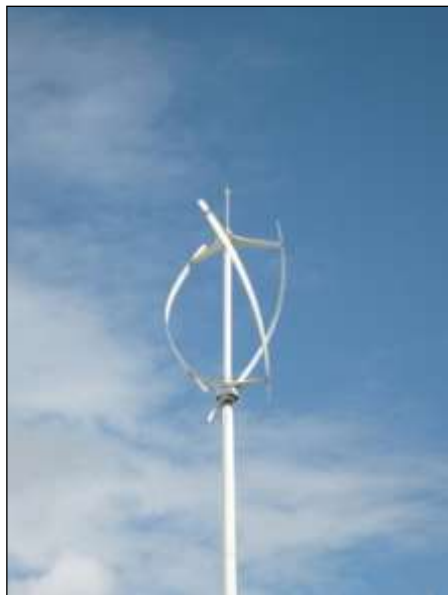
Figure 5 Soak testing the completed turbine
