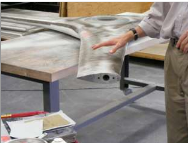
Figure 3 Carbon Fibre base unit for blades
