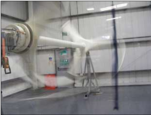
Figure 5 Soak testing the completed turbine
